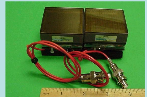
A pair of Hamamatsu H8500 square face (52 mm x 52 mm) Position Sensitive Photomultiplier Tubes (PSPMTs)
